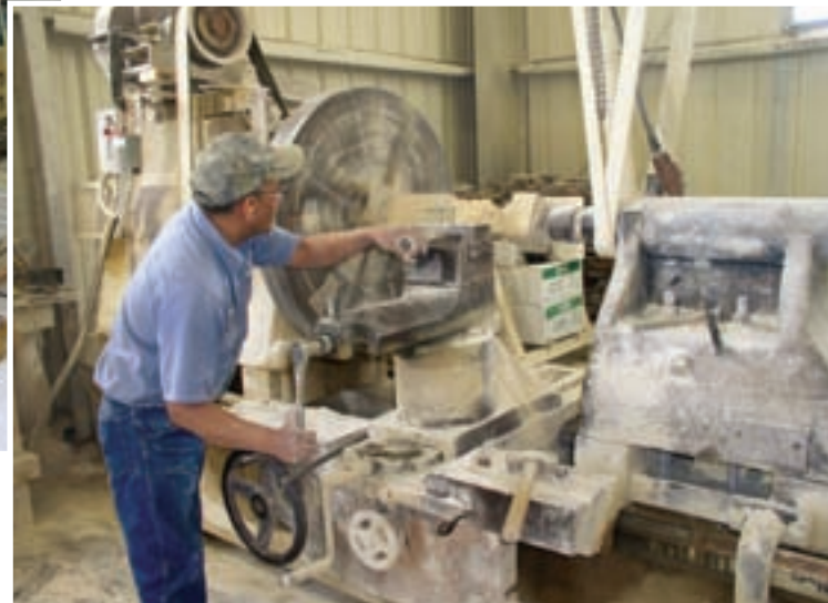
Three stone lathes are used for turning columns and balusters.
