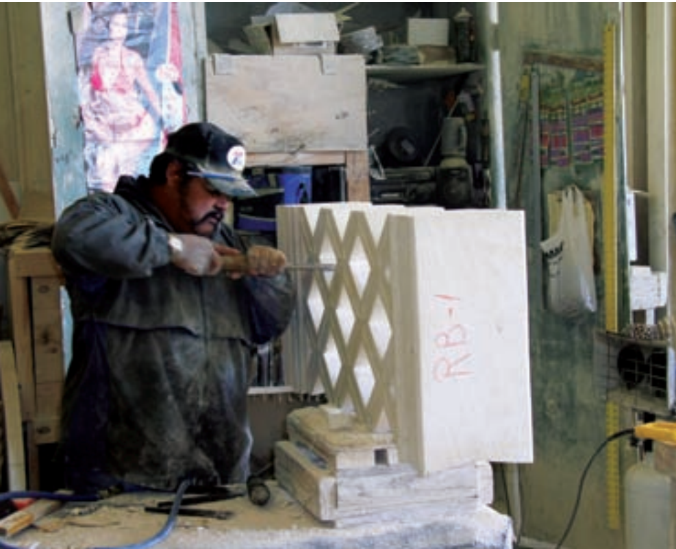
At the mill, skilled workers use hand tools to carve detailed limestone pieces.
