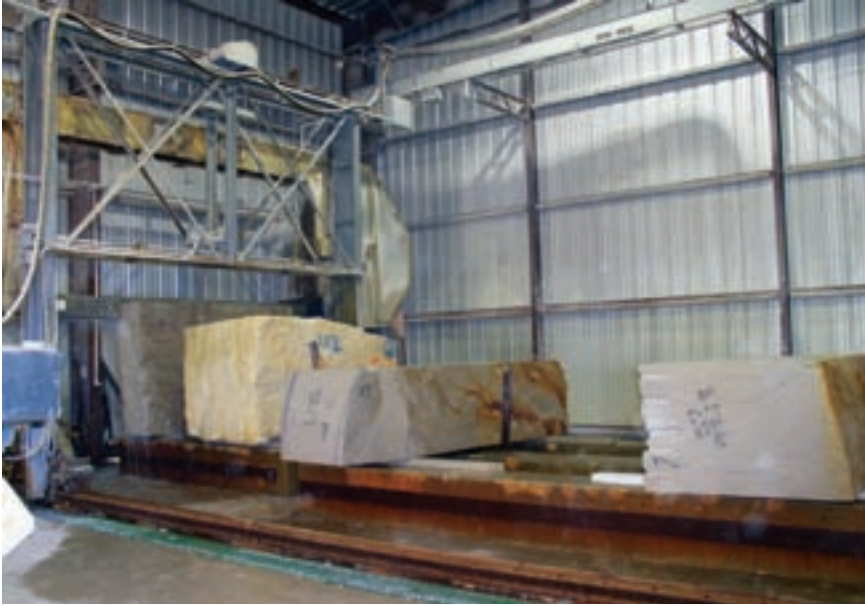
The fabrication process begins with blocks being cut by a 15-foot diamond belt saw.
