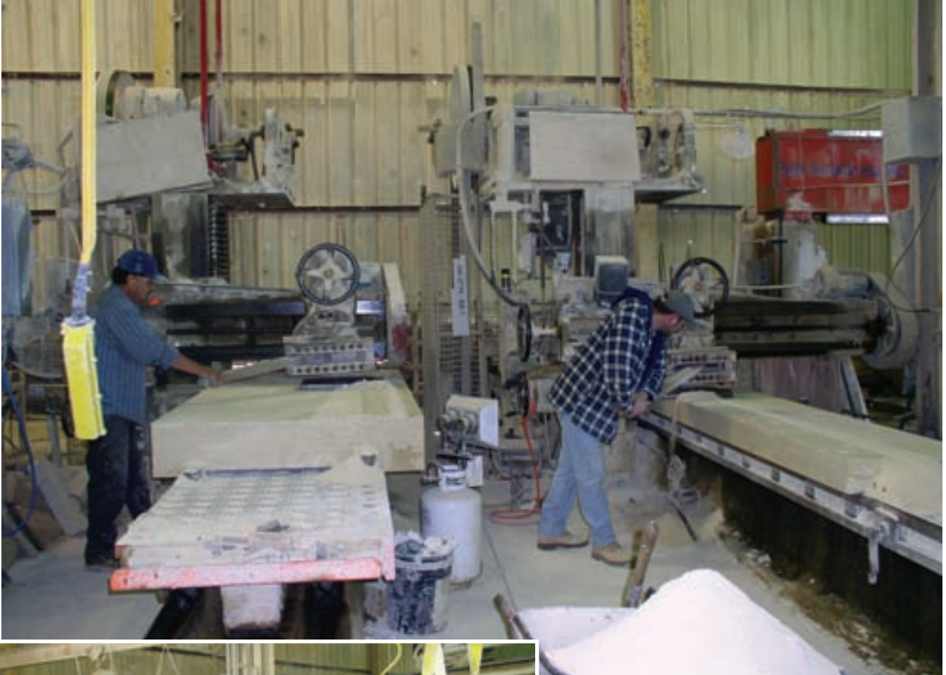
The planers are instrumental in smoothing limestone slabs and ensuring that they are all consistent in size.
