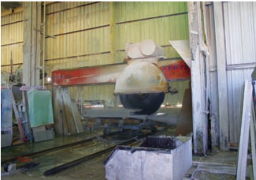
A 72-inch FB72-11 fixed bridge saw from Park Industries of St. Cloud, MN, is also in place to cut limestone pieces.
